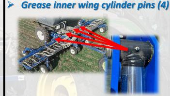
Grease Inner Wing (4) and Outer Wing (4) Pivot Pins
