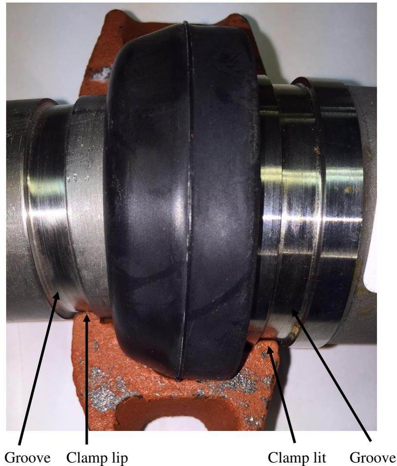
16. Install the second clamp, bolts and nuts as shown below. The clamps must be touching for the clamps to seal completely.
